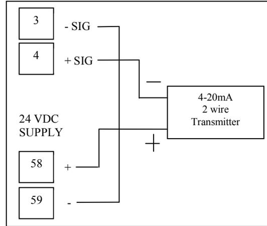
**0-20mA Transmitter Wiring Diagram**
