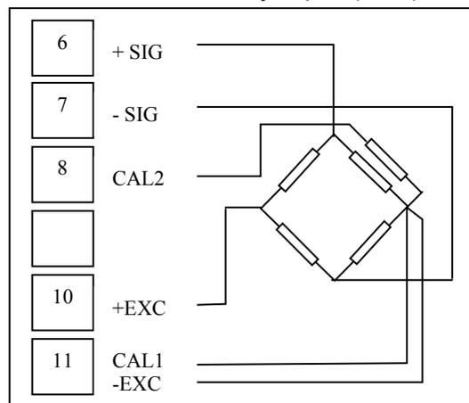
Note: If no internal Rcal is used, Cal1 and Cal2 may be omitted. For transducers with External cal resistors, please refer to the manufacturers recommended wiring instructions.
