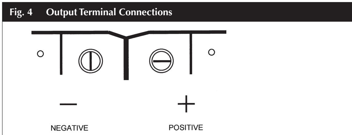
A load resistor, typically 250 ohms, may be connected in series with either terminal of the transmitter. For Digital communications, 250 ohms must be connected in the loop. The maximum series resistance in the circuit (including wiring lead resistance) can be calculated using the formula:
