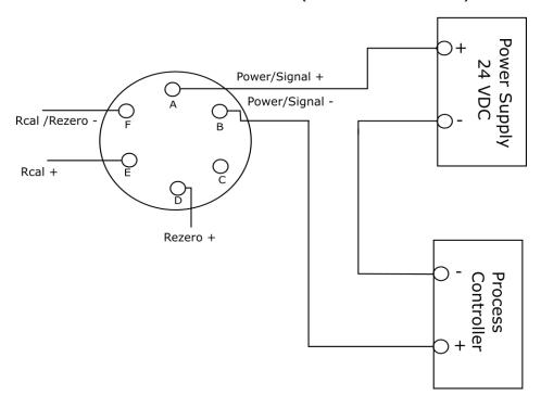
4-20 mA WITH GUARDIAN RELAY WIRING EXAMPLE (8-PIN CONNECTOR)
