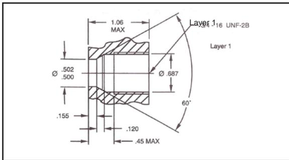
Figure 1: PT375 Mounting Hole Diagram
