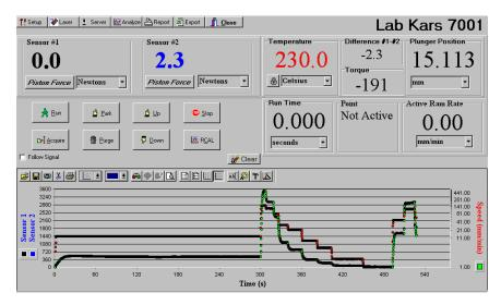
**Control Buttons** The rheometer crossbar and test run can be controlled manually from the operation buttons at the top of the rheometer control page.
