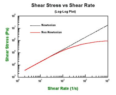
The Newtonian region for materials on a log-log plot of shear stress vs. shear rate is where the slope is equal to 1.0. For most polymers, the slope falls to less than 1.0 as the shear rate increases.
