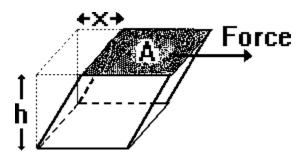
Shear Stress =  $\tau$  = Force / Area = F / AShear Strain =  $\gamma$  = Displacement / Gap = x / hStrain Rate =  $\mathcal{R}$ =Displacement Rate / Gap =  $x \mathcal{R} h$
