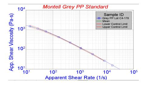
Repeat steps 3 - 4.12 three times. Data will be logged for both sensors. All 3 curves should lie within the SQC tube.
