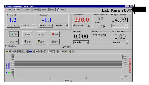
If you need to change the version of LabKARS you are working with, click on the Reports Icon in the tool bar at the top of the page. In the upper Left hand corner of the Reports screen, change the Model Number and Serial Number to the rheometer you are working with then click on the Update button to the right. Be sure to close down and Restart LabKARS to refresh the system after you have made your changes.
