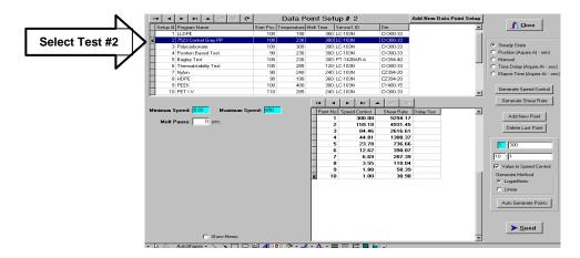
Verify that the data points are setup to perform 10 Data Points from 300 mm/min to 1 mm/min in a logarithmic sequence. (See Figure 2.1 for actual settings)
