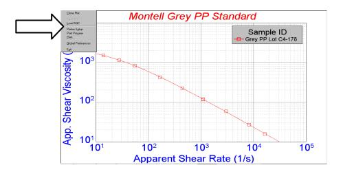
Choose the SQC ID that applies to the test and the material sample used to test the rheometer. In this case Profax 7523 @ 230C with the X300-33 Die.
