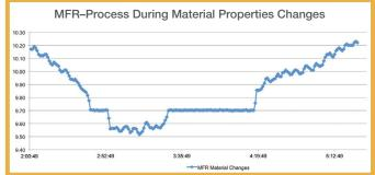
The above graph shows process readings taken by the ViscoSensor during material processing that is in flux. The stock material has fundamentally changed or a contaniment has entered the process. For example, the flux could be a result of a change in molecular weight/branching or a different material grade being mixed in. The process metric was recovered by addressing the cause of the change measured by the ViscoSensor.
