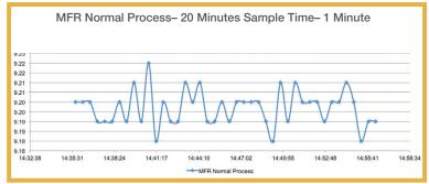
The above graph shows process readings taken by the ViscoSensor during relatively consistent material processing. With consistent Melt Flow Ratio (MFR), one knows the material is homogenous as well as molecular weight concluding that polymer chain branching is staying constant.
