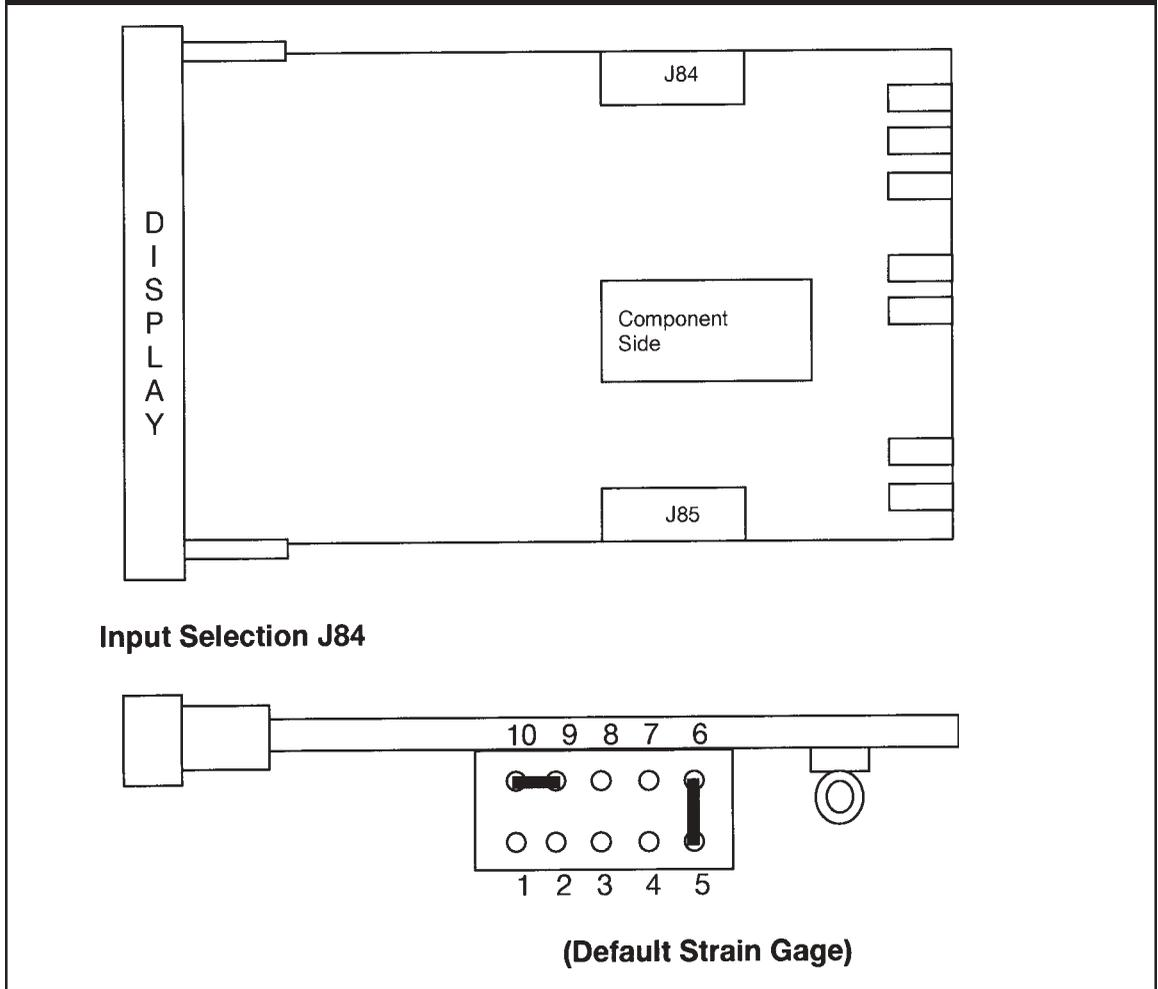
**6.1.2 SETTING THE SHUNT CALIBRATION FOR STRAIN GAGE TRANSDUCERS AND AMPLIFIED TRANSMITTERS**
