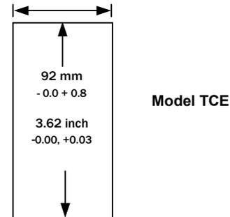
**1.4.3. Recommended Minimum Spacing of Controllers.**
