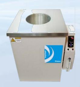
Dynisco's PolyClean is a fluidized temperature bath that will clean parts and tooling 2 to 3 times faster and safer than traditional cleaning method, such as an oven. Our fluidized bath system is aircontrolled with advanced PID temperature controller for optimal thermal performance. The system uses aluminum oxide sand (heated up to 1112°F) and air to surround the part or tooling. The "sand" will gently breakdown the polymer without damaging the part or tooling.
