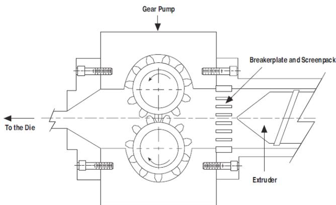
Figure 3. Gear Pump
