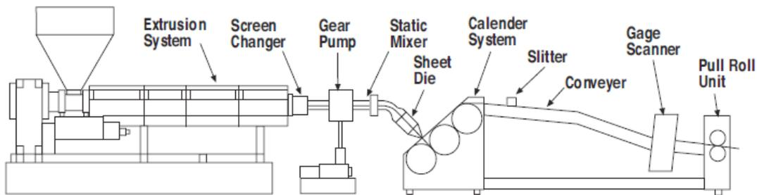
**Figure 6. Sheet and Film Extrusion**
