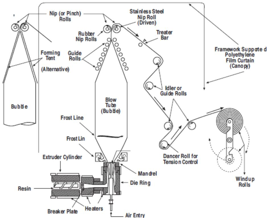
Figure 5. Blown Film Extrusion
