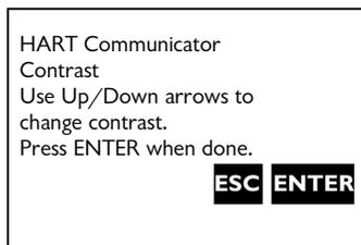
2. Follow the on-screen instructions to adjust the display contrast. Press **ESC** (F3) to return to the configure Communicator Menu without adjusting the contrast. To save the changes to the contrast, press **ENTER** (F4) and the Configure Communicator Menu appears. **ENTER**
