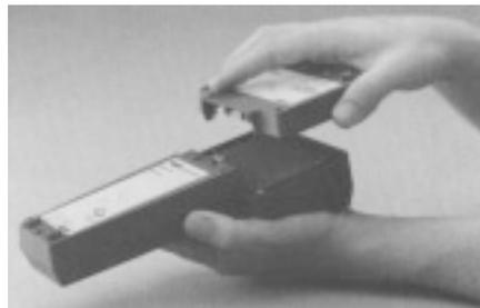
1. Completely loosen the three captive screws holding the communicator battery pack.
