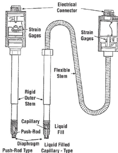
Figure 32a. Pressure Transducers
