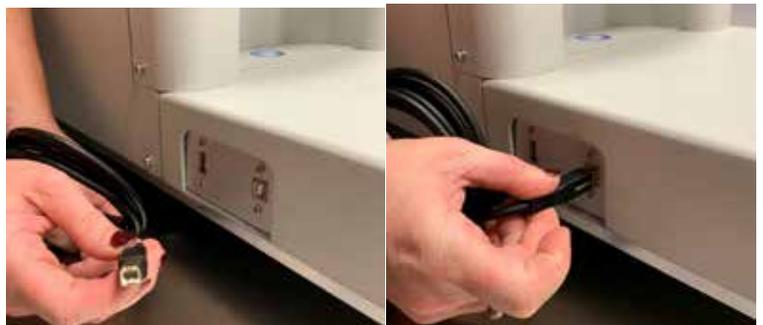
Step 14: Connect the other end of the USB Cable into the Instrument
