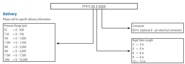
Mating connector P/N711600 or 6 - pin cable assembly for B314 option sold separately.
