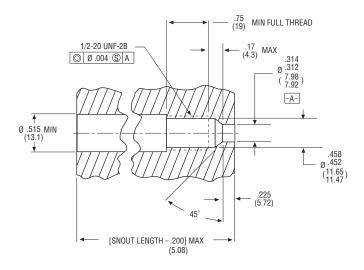
All dimensions are inches (mm) unless otherwise specified. ©2016. Dynisco reserves the right to make changes without notice. Refer to www.dynisco.com for access to Operator Manual and other support documentation. DSMDT4X2FSIL2 Rev: 1216
