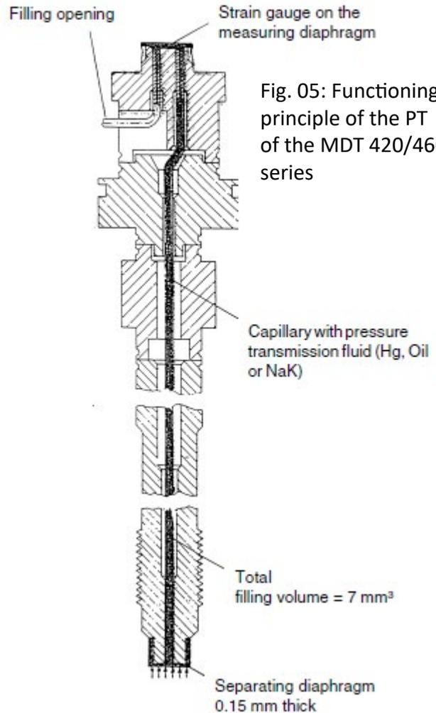
Fig. 05: Functioning principle of the PT of the MDT 420/460 series
