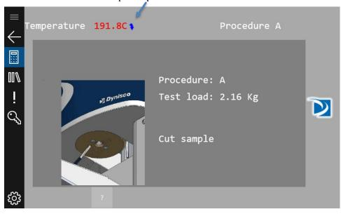
For each sample cut, the LMI will either cut (or prompt the user to cut) the sample after the sample time interval has elapsed. Ensure that the samples are moved away from the landing area, so samples don't fuse together.
