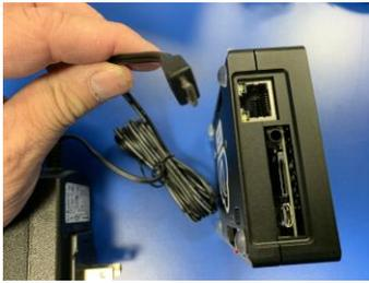
Step 7: Locate Power Connection on Dynisco Edge Device
