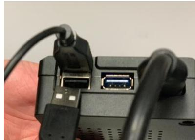
Step 12: Insert USB Cable (Keyboard/Mouse) Into Dynisco Edge Device
