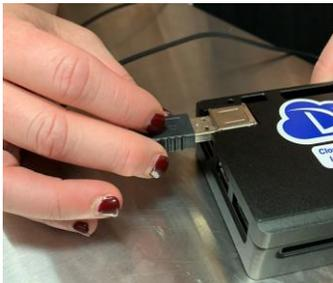
Step 9: Insert USB Cable into the USB2.0 Slot on the Dynisco Edge Device Shown Above
