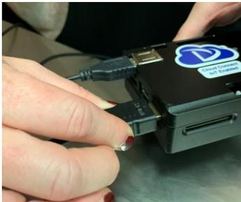
Step 11: Insert HDMI Cable for Computer Monitor (Both Customer Supplied) into the Dynisco Edge Device
