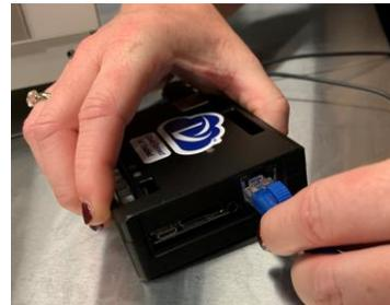
Step 10: Insert Ethernet Cable (Customer Supplied) into the Dynisco Edge Device
