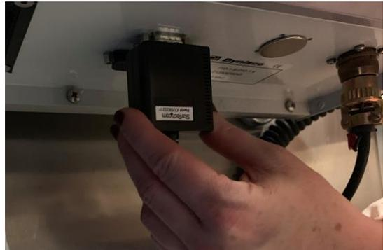
Step 15: When you See this Prompt, Connect the Serial end of the USB Cable into the Instrument and Click OK
