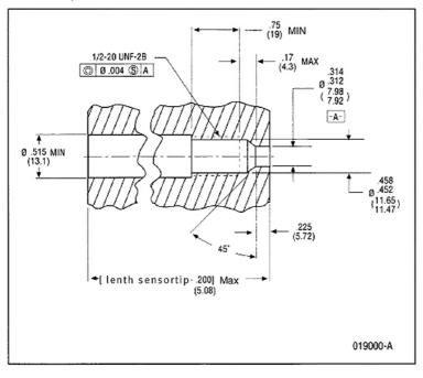
Melt temperature sensor with ½-20 UNF thread
