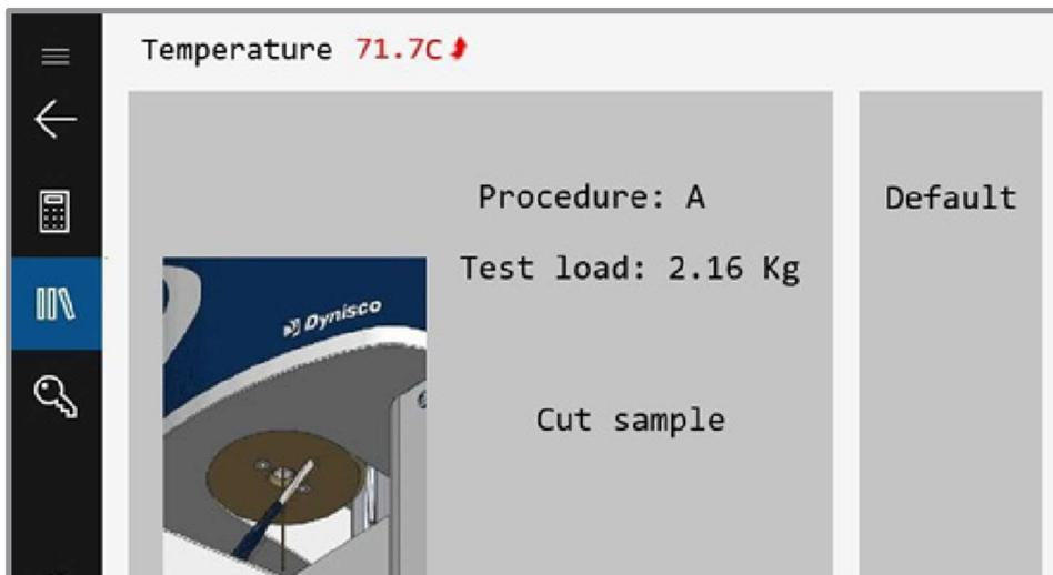
For each sample cut, the LMI will either cut (or prompt the user to cut) the sample after the sample time interval has elapsed. Ensure that the samples are moved away from the landing area, so samples don't fuse together.
