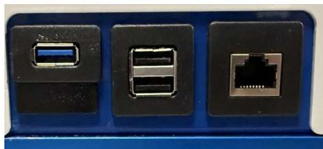
On the right side of the LMI there are three USB ports and one Ethernet port.
