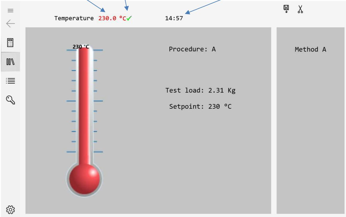
Once the LMI is at the setpoint temperature, a 15-minute count-down timer will start. Ensure that the piston and die are in the unit. After this timer expires, the LMI will be ready to load with material as shown below:
