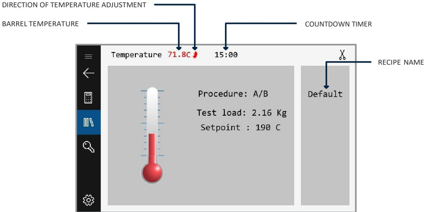
Once the LMI is at the setpoint temperature, a 15 minute count-down timer will start. Ensure that the piston and die are in the unit. After this timer expires, the LMI will be ready to load with material as shown below:
