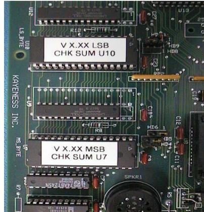
Remove the USB and LSB by gently prying loose with a flat-blade screwdriver. Begin prying the firmware ICs from left side switching from left to right side to extract the firmware IC evenly. This will prevent socket damage and bent firmware IC leads.
