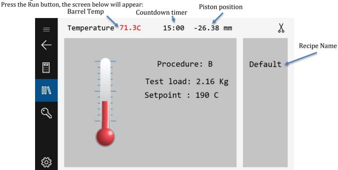
Once the LMI is at the setpoint temperature, a 15 minute count-down timer will start. Note that the timer will only appear if the recipe is set to "ASTM" mode, if operating in ISO mode, the user is not required to wait for the 15 minute stabilization timer, and can simply tap at any point to begin the test. *Ensure that the piston and die are in the unit.* After this timer expires, the LMI will be ready to load with material as shown below:
