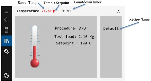
Once the LMI is at the setpoint temperature, a 15 minute count-down timer will start. Note that the timer will only appear if the recipe is set to "ASTM" mode, if operating in ISO mode, the user is not required to wait for the 15 minute stabilization timer, and can simply tap at any point to begin the test. *Ensure that the piston and die are in the unit.* After this timer expires, the LMI will be ready to load with material as shown below:
