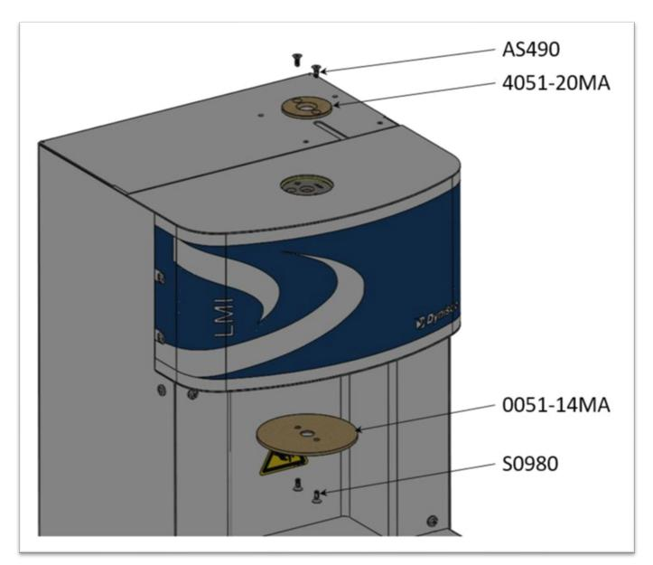
CAUTION: Parts identified above can be replaced by user. First turn off unit, disconnect power and allow unit to cool to room temperature before replacing.
