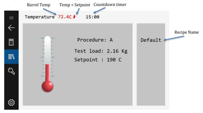
Once the LMI is at the setpoint temperature, a 15 minute count-down timer will start. *Ensure that the piston and die are in the unit.* Note that the timer will only appear if the recipe is set to "ASTM" mode, if operating in ISO mode, the user is not required to wait for the 15 minute stabilization timer. After this timer expires, the LMI will be ready to load with material as shown below:
