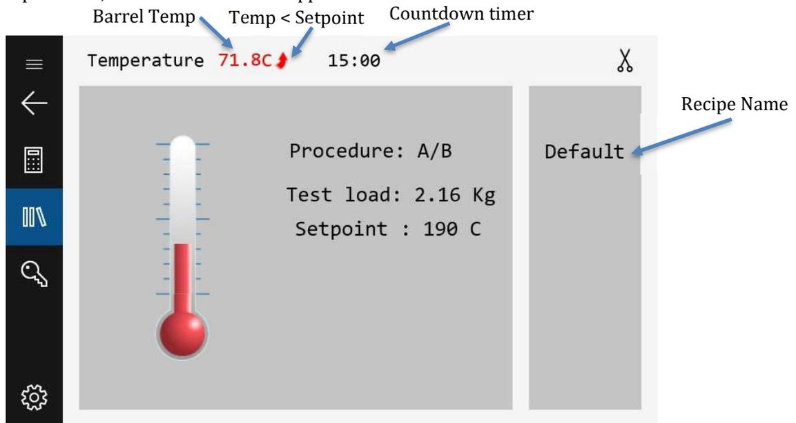
Once the LMI is at the setpoint temperature, a 15 minute count-down timer will start. *Ensure that the piston and die are in the unit.* After this timer expires, the LMI will be ready to load with material as shown below:
