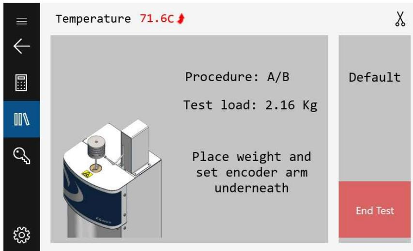
Press the screen again when loading is complete. The melt-time will be displayed on the screen as shown below:
