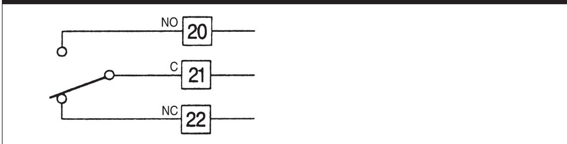
**Fig. 11 Alarm 2 Relay Wiring**
