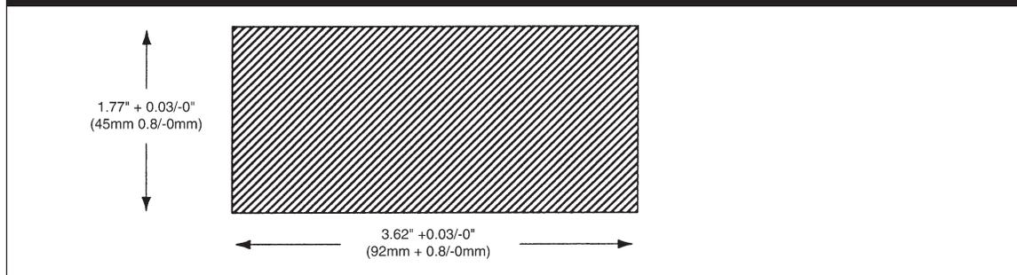
HORIZONTAL MOUNTING: Minimum distance between cutouts: 20 mm
