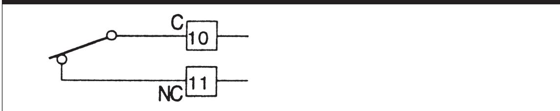
The relay output is an SPST relay, without snubber network.
