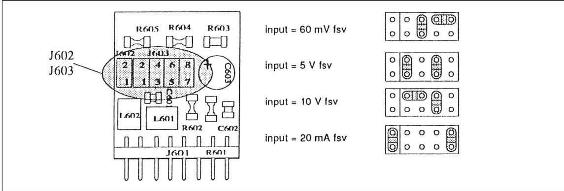
2) The instrument is shipped with a 20mA (  standard) analog retransmission (when fitted). When it is desired to use a 10 V analog retransmission, the solder jumpers should be set properly in accordance with the table below.
