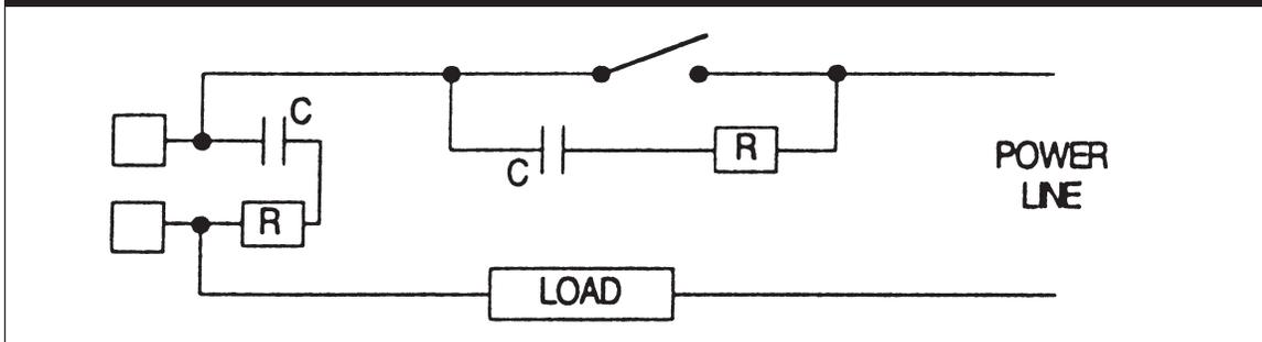
In this case it should be better to protect the switch also as shown in Fig. 14. Anyway the cable involved in relay output wiring must be as far away as possible from input or communication cables.
