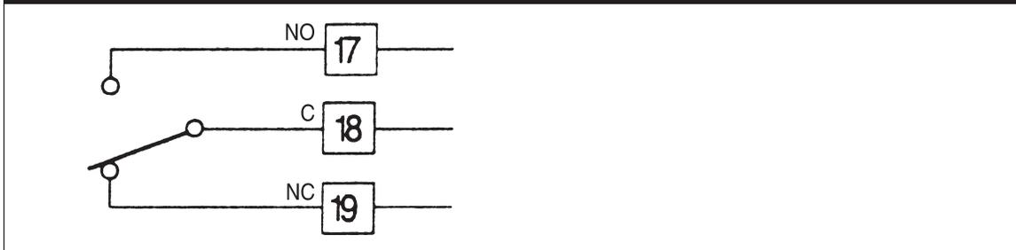
The relay output is an SPDT relay, without snubber network.
