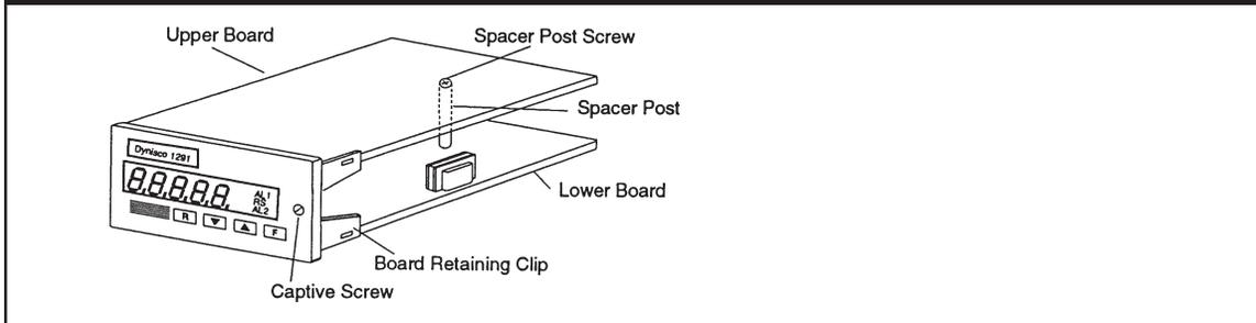
3. Using your fingers, gently pull the plastic board retaining clips away from both printed circuit boards on one side until they pop free. Then, release the other side.
