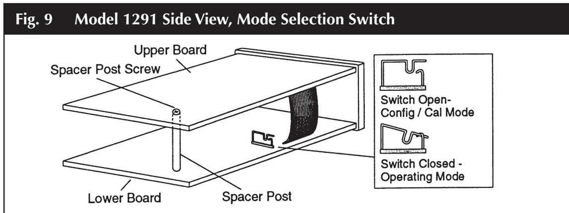
To access the Mode Selection Switch slide out the front panel and printed circuit board assembly, as instructed by steps 1 and 2 of Disassembly on page 15. Refer to Figure 9 to locate the switch and change the setting. Once the switch is set, go to the following Reassembly procedure. Skip steps 1-5 if the unit was not disassembled.
