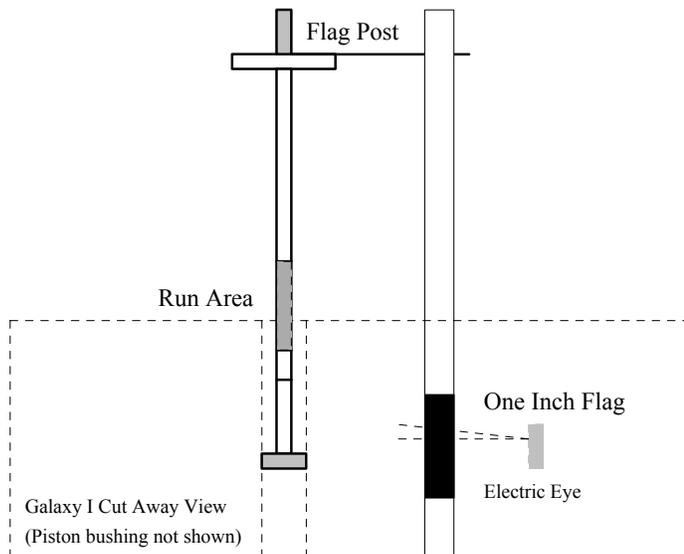
Plunger for Method B and Method A/B Measurements
