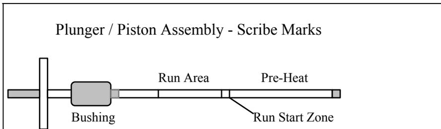
After melt time (pre-heat) is completed, and after the piston lowers into the "run area" as denoted by the scribe marks on the piston assembly, make a
