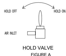
4.) Confirm that the hold valve switch is in the HOLD OFF position. See figure A.
