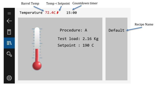
Once the LMI is at the setpoint temperature, a 15 minute count-down timer will start. *Ensure that the piston and die are in the unit.* After this timer expires, the LMI will be ready to load with material as shown below:
