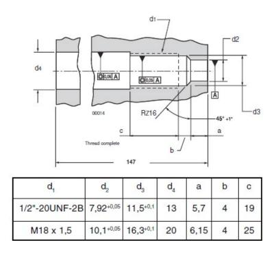
Fig. 07: Mounting hole for transmitter MDT467  $\boldsymbol{x}$
