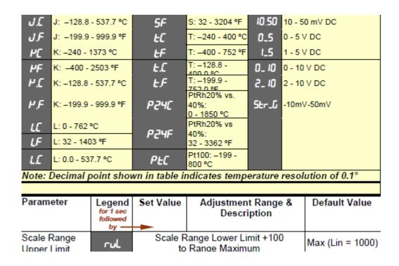
The "ruL" should match the upper range of the pressure sensor being used
