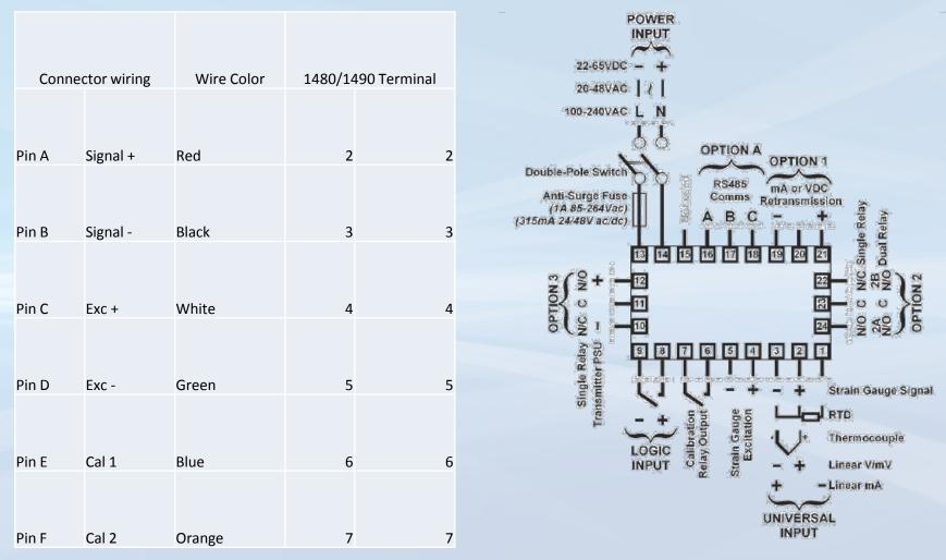
Wiring for strain gauge pressure transducer, mV output
