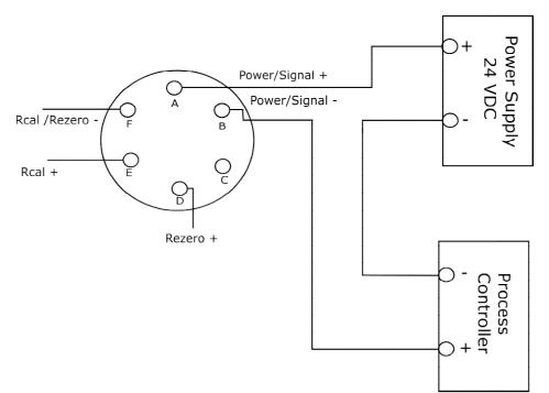
4-20 mA WITH GUARDIAN RELAY WIRING EXAMPLE (8-PIN CONNECTOR)
