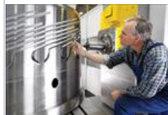
This pipe distributor from KM-Berstorff is part of a line built to produce pipe up 95-in. diam.
