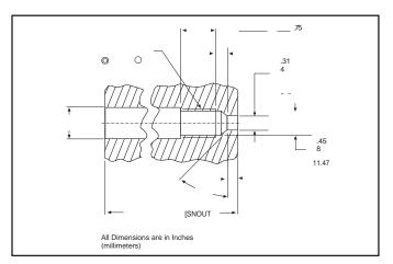
1/2-20 UNF Mounting Hole Diagram
