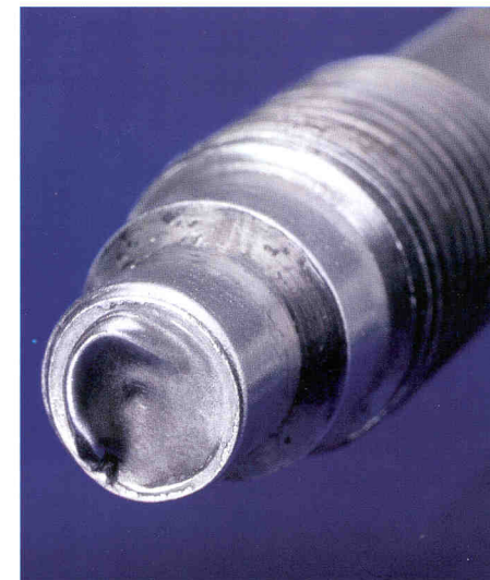
Transducer damage caused by mis-machined hole.
